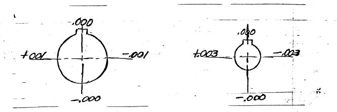
At no time should a crankshaft, which is found to be bent, be straightened.
